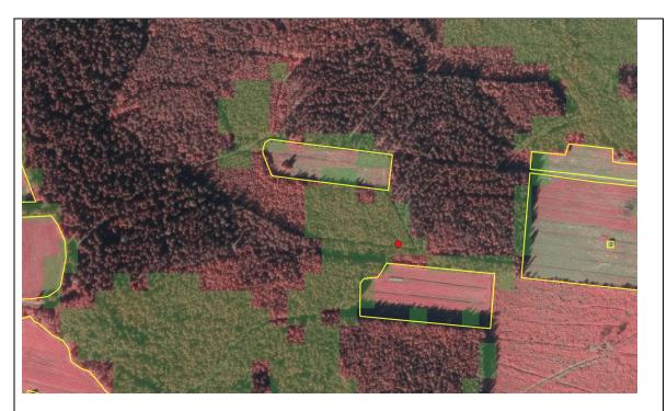
**Fig. 6** Commission error on broadleaved dominated class. HRLclassification showing broadleaved dominance (green raster), overlaid over aerial imagery. Ground truth data measured on the plot (red dot) indicates coniferous dominance. Yellow delineation indicates agricultural fields (7040053, 505030).
